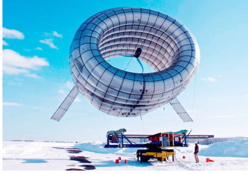
Figure 1: Altaeros Buoyant Airborne Turbine (BAT), Image Credit: [5]
